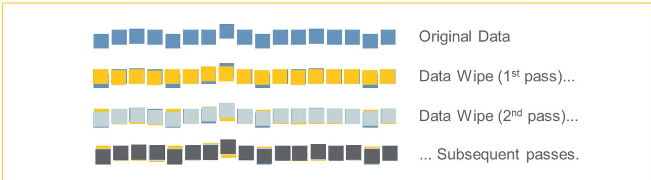
*Fig. 4. Demonstrating the data-wiping process through multiple passes of over-writing*
